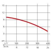
The diagrams show you the pumping capacity of the Rössle submersible pumps in m³ per hour in relation to the pumping height.
