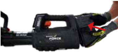
Figure 4: First press the IP 68 battery cover on at the top edge of the housing
